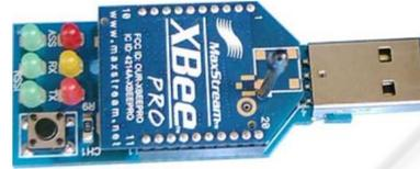
Figure 5: USB interface board.
