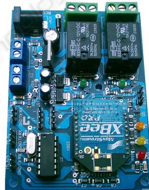
Figure 6: Sensor and actuator board.
