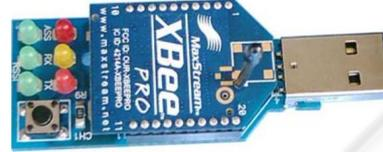
Figure 5: USB interface board.
