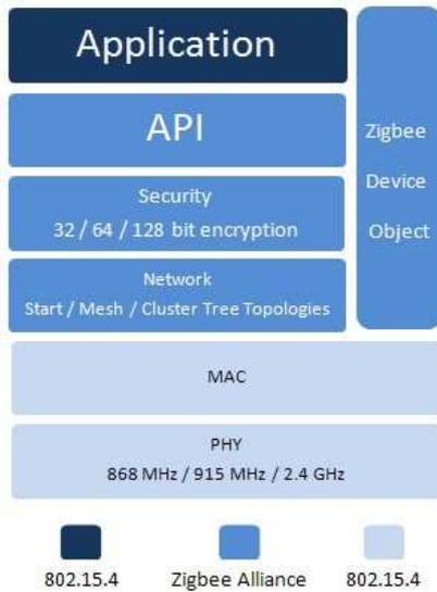
Figure 2: ZigBee stack architecture.
