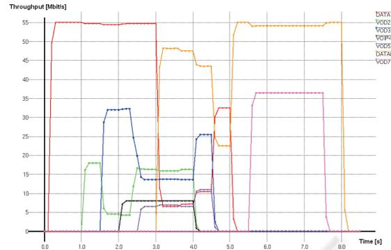
Figure 2: Throughput of particular flows with implementation of MAM model.
