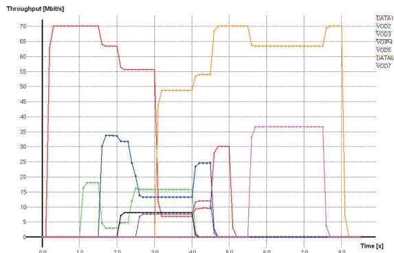
Figure 3: Throughput of particular flows with implementation of RDM model.
