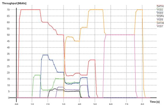
Figure 1: Throughput of particular flows without utilization of QoS mechanisms.
