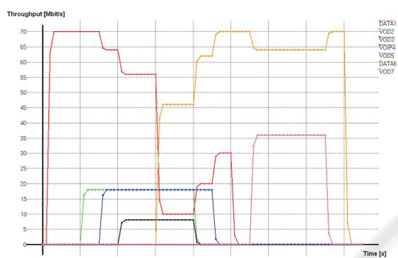
Figure 4: Throughput of particular flows with implementation of RDM model and Measured Sum method for VoD traffic.
