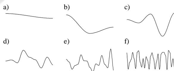
Figure 4: Octaves that are added to the final 1D Perlin noise with the same amplitude and different frequencies: a) 1, b) 2, c) 4, d) 8, e) 16, f) 32.
