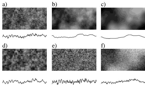
Figure 5: 2D Perlin noise after summing up 6 noise functions with different amplitudes. Amplitude of each following octave is a) the same; b) half; c) quarter the size. d-f) Perlin noise generated according to three different amplitude vectors.
