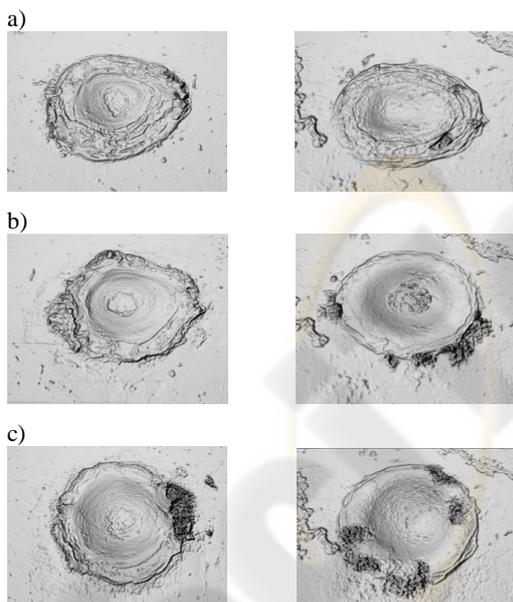
Figure 10: Real and generated samples: a) 10; b) 50; c) 100 laser pulses burned into a single point in steel.
