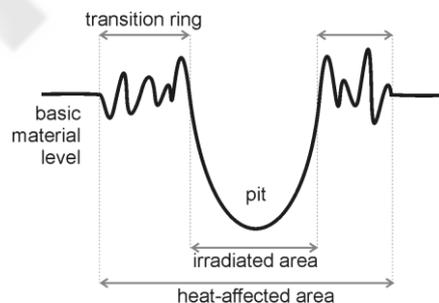
Figure 1: A typical cross-section of a sample.
