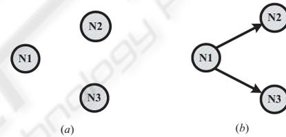
Figure 2: (a) Three isolated nodes. (b) Star coupled network with master node  $N1$ .
