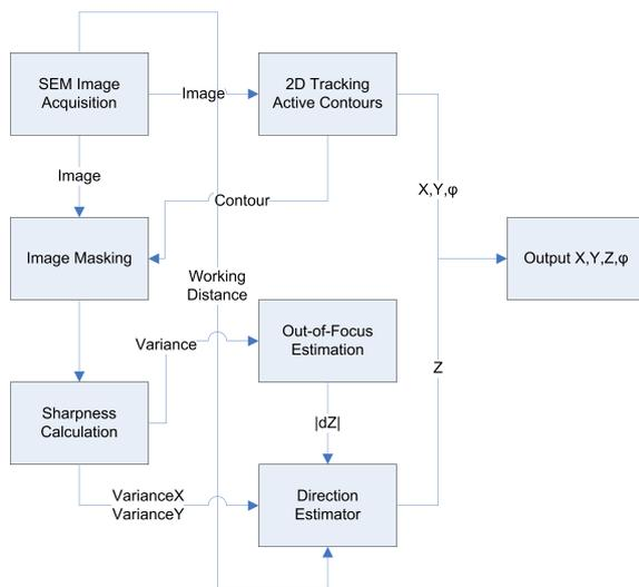
Figure 7: The complete 3D tracking algorithm in the initial state.
