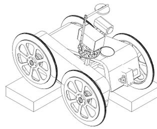
Figure 4: Joint suspension system of the robot.
