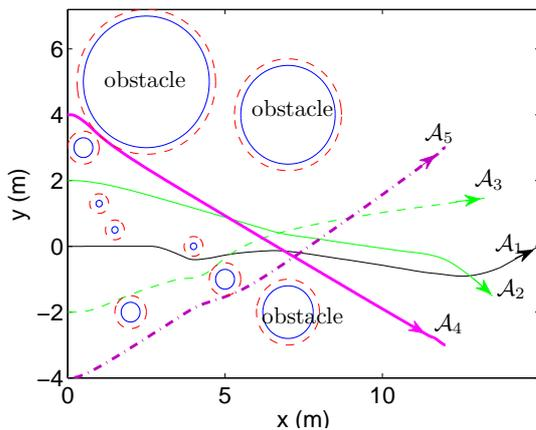
Figure 6: Collision avoidance of five robots.
