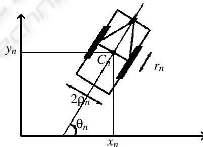
Figure 2: Unicycle-type robot.
