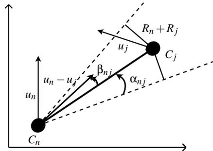
Figure 3: Velocity obstacle concept.
