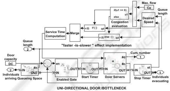
Figure 2: *SimEvents* implementation of bottlenecks.
