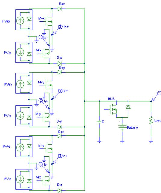
Figure 1: Sequential Shunt Regulator.
