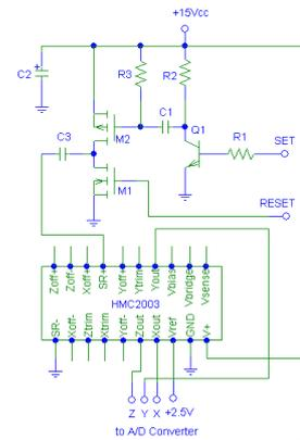
Figure 8: Magnetometer circuit.
