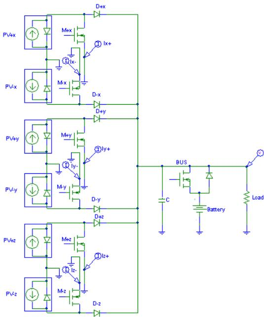
Figure 1: Sequential Shunt Regulator.
