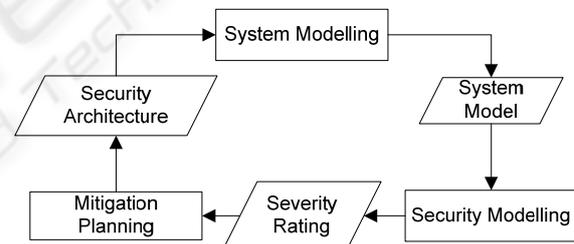
Figure 1: The cyclic security assessment process defined by the ESSAF method aims at refining design architectures and revising security implementations.
