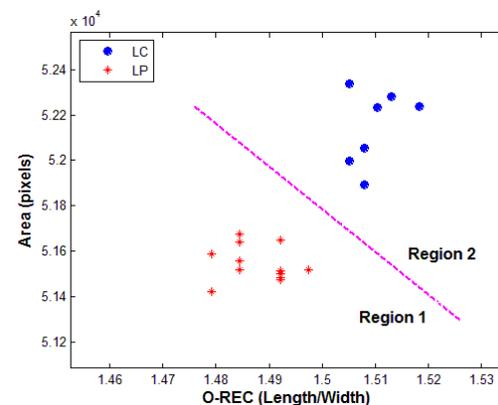
Figure 8: Separating LC and LP Dish Types.
