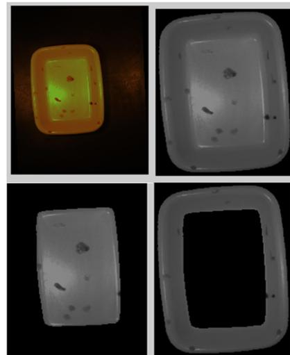
Figure 9: Partitioning process (SC Dish): Original Camera Image (top-left), Gray Scale Pre-processed Dish Image (top-right), Dish Floor Region (bottom-left), and Dish Wall Region (bottom-right).
