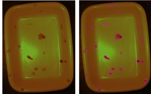
Figure 12: Original SX (left) and All Dirt Spots Detected (right).
