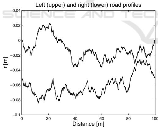
Figure 2: Two tracks across an "average" isotropic surface.
