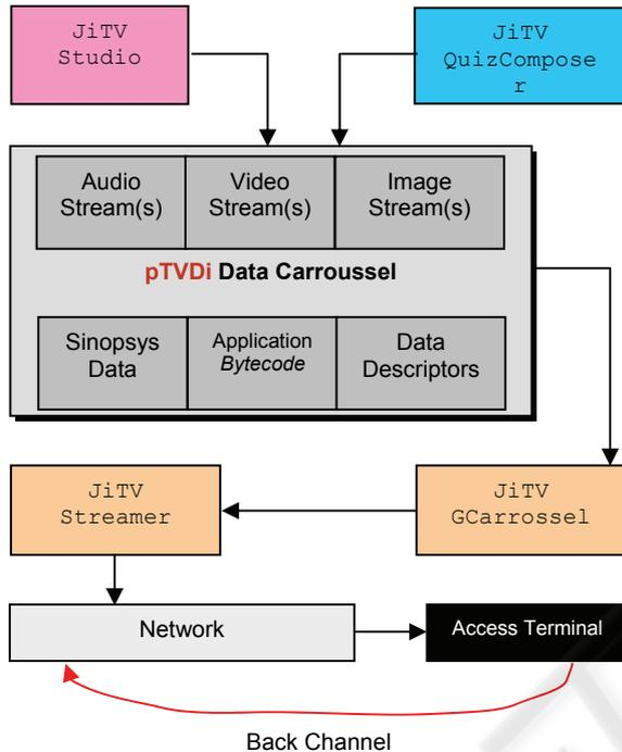
Figure 3: Architecture of the JiTV Platform (production, distribution, interaction and back channel).
