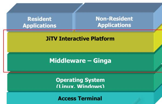
Figure 1: Architecture of the JiTV Platform.
