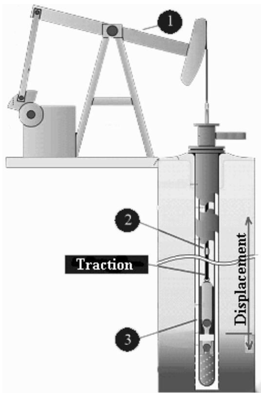
Figure 1: The Pump Mechanical System.
