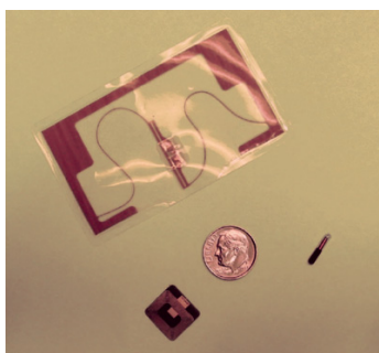
Figure 4: Different shape and sizes of RFID Tags (Want, 2007).
