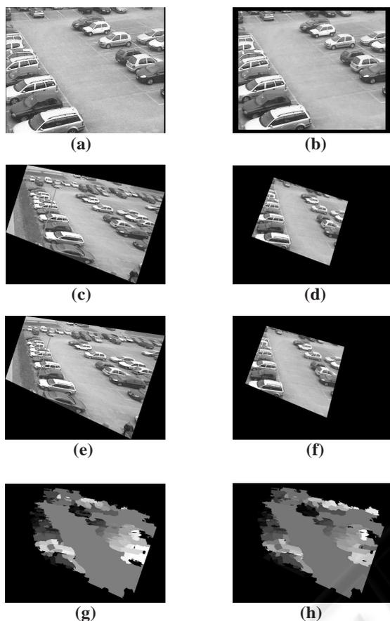
Figure 5: Results for a pair of stereo images having focal ratio 0.90. Heterogeneous right image (a); homogeneous right image (b); heterogeneous pair of rectified images (c & d); homogeneous pair of rectified images (e & f); range image using heterogeneous rect. pair of images (g); range image using homogeneous rect. pair of images (h). Left image of input stereo pair is same as in Figure 1(a).
