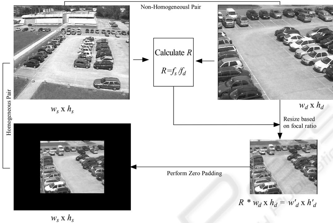
Figure 1: Overall process to obtain the pair of homogeneous images.
