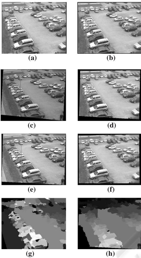
Figure 3: Results for a pair of stereo images having focal ratio 0.97. Heterogeneous right image (a); homogeneous right image (b); heterogeneous pair of rectified images (c & d); homogeneous pair of rectified images (e & f); range image using heterogeneous rect. pair of images (g); range image using homogeneous rect. pair of images (h). Left image of input stereo pair is same as in Figure 1(a).
