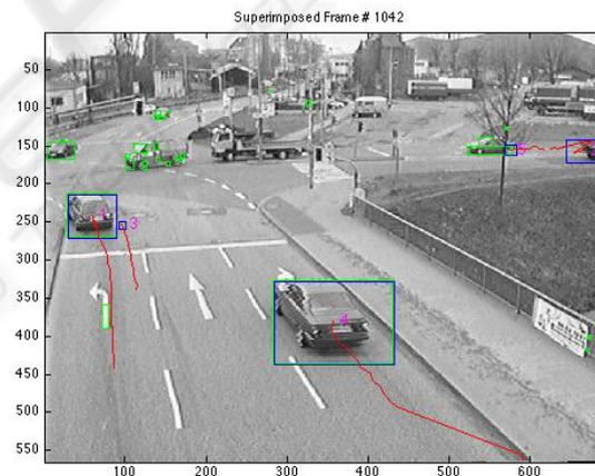
Figure 4: Tracking of various moving vehicles.
