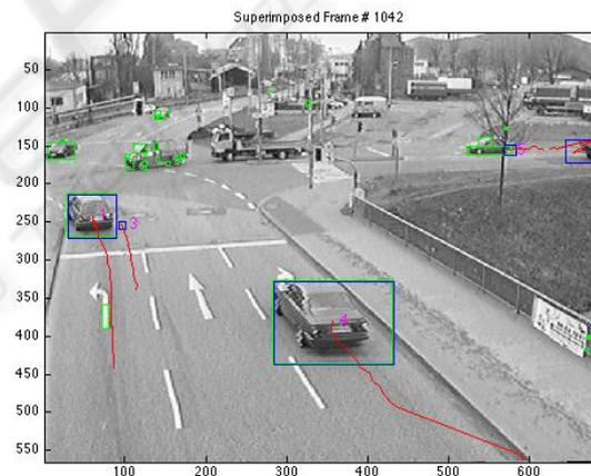
Figure 4: Tracking of various moving vehicles.
