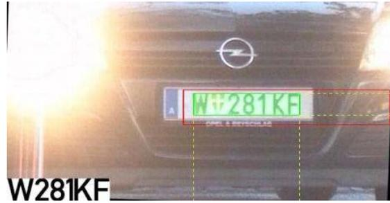
Figure 11: Correctly identified plate although the lights of the car influence the segmentation.
