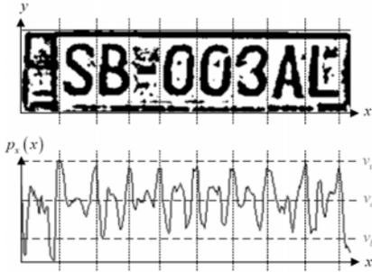
Figure 7: Segmentation using the vertical edge projection from (Martinsky, 2005).
