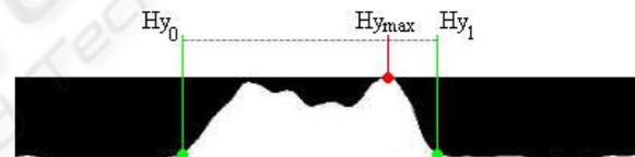
Figure 4: Boundary detection of the edge projections.
