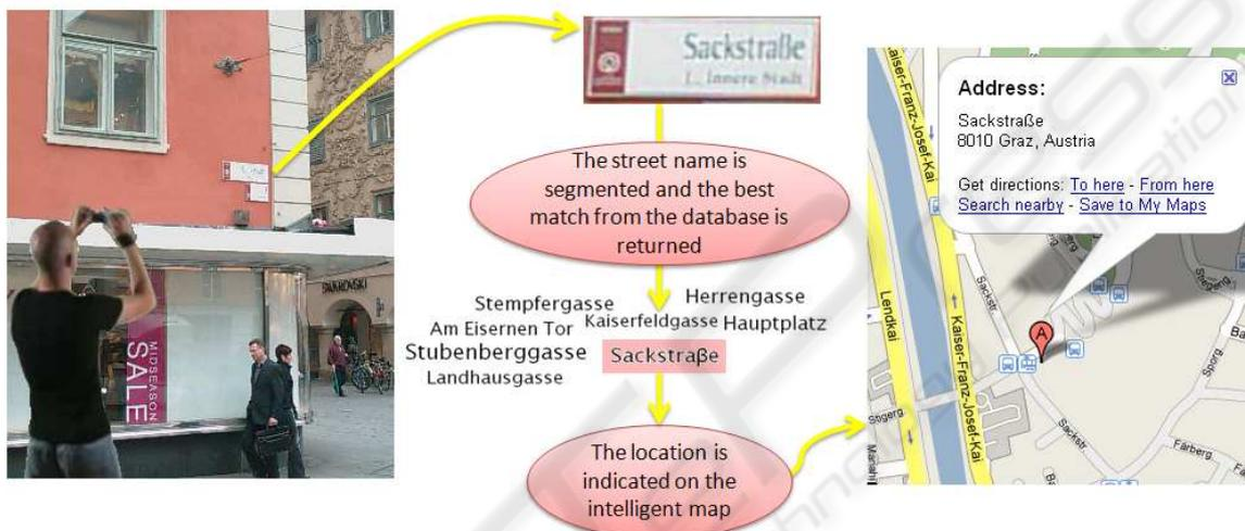
Figure 3: User takes an image from an urban place using his/her mobile phone and sends it to a server. Some target objects within the image are detected (the street plate) such that location of the person can be identified by recognizing some uniquely discriminant sign within the detected area of interest (the street name).
