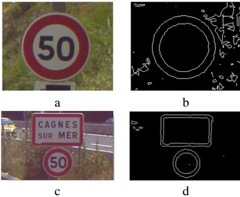
Figure 7: Image of a road sign (a,c) and contour detection (b,d).
