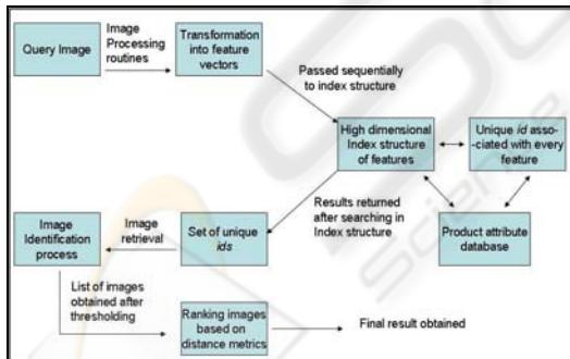
Figure 1: A basic query processing model.
