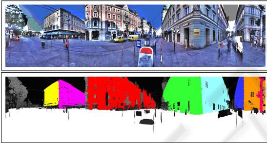
Figure 3: Top: Laser RGB texture (shading corrected) in spherical coordinate system, Bottom: Plane (colored) segmentation using RANSAC.
