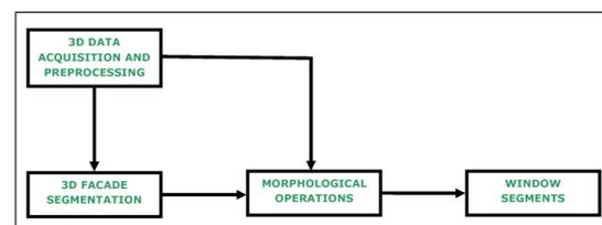
Figure 2: Pipeline for window detection from a 3D laser spherical coordinate system image, or optionally using ortho images from 3D Facade segmentation which facilitates the window detection process.
