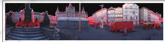
Figure 4: RGB image of urban scene in spherical laser scanner coordinates, overlaid by a binary mask from thresholding that resembles window candidate pixels.
