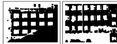
Figure 5: Closing joins the separate portion of the windows to be considered as a single window for the detection framework, examples from facades ortho images.
