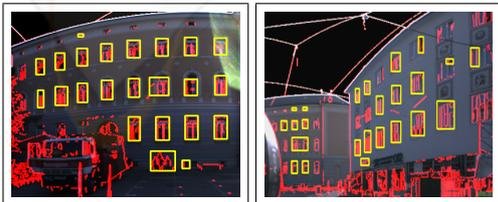
Figure 6: (a), (b) Examples for Window Segments detected by the system on the laser spherical coordinate system image.
