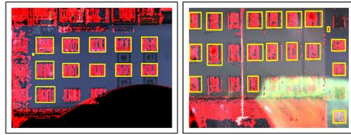
Figure 7: (a), (b) Examples for Robust Window Segments detected by the system on the ortho images of segmented 3D facades.
