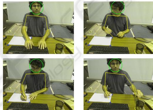
Figure 5: Tracking samples of a sequence where the subject types something in the keyboard, picks a pen, writes and leaves the pen again. The tracker is able to recover the pose after several errors due to fast apparent motion.
