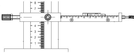
Figure 4: One of the “2D Positioner” and the vertical piece of the body of the instrument.
