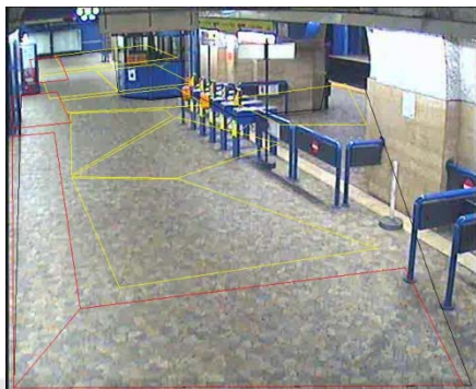
Figure 4: The yellow polygons show the outline of the learned lost zones. The red polygons show the outline of the entry zone, exit zone and IO zones.
