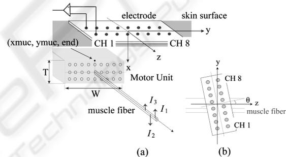
Figure 2: Illustration for the SEMG generation model. (a) Spatial relation between the electrode and the muscle fiber; (b) Electrode angle  $\theta$ .
