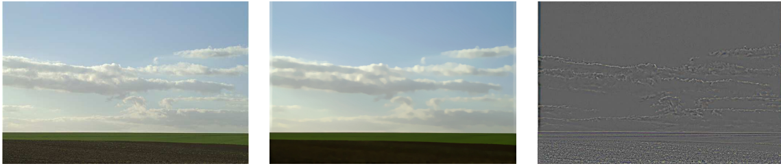
Figure 1: Result of the structure/texture decomposition algorithm from (Vese and Osher, 2003). The first column shows the original image, the second column the structure image, and finally the last one the texture image.
