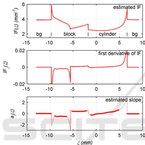
Figure 6: Estimated IF, and its derivative together with the estimated slope of the profile.
