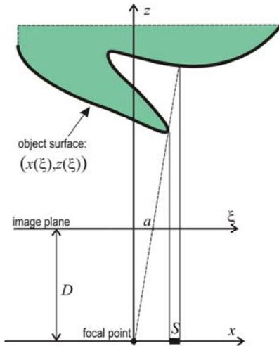
Figure 2: Camera and Scene geometry.
