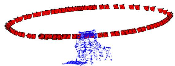
Figure 3: Point cloud for the sequence *House* together with the camera trajectory.
