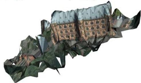
Figure 8: Two colormap views of the mesh and view of the textured reconstruction produced from the sequence *Gottesau* by the conventional-spline-based procedure. The original point cloud is indicated by green points.
