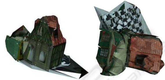
Figure 7: Two views of the triangular mesh and two views of the textured reconstruction from the sequence *House* produced by the conventional-spline-based procedure.
