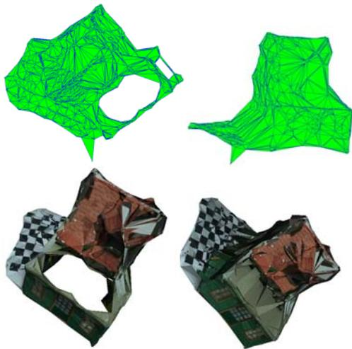
Figure 9: Two views of the mesh and of the textured reconstruction produced from the sequence *House* by the  $\alpha$ -shapes procedure. Left  $\alpha = 1.0 \cdot 10^4 \sigma$ , right  $\alpha = 2.0 \cdot 10^4 \sigma$ .
