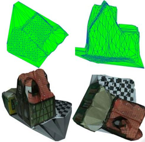
Figure 5: Two views of the triangular mesh and two views of the textured reconstruction produced from the sequence *House* by the  $L_1$ -spline-based procedure.
