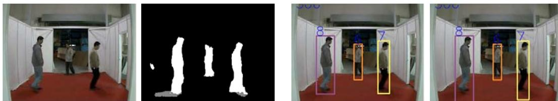
Figure 1: From left to right, the first figure is original image. The second one is foreground with foreground as white and shadow pixels as grey. The last two compares the accuracy of object tracking with and without shadow removing respectively.
