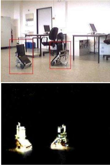
Figure 1: Results of the background subtraction.
