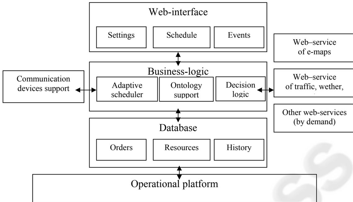
Figure 1: Architecture Of Systems For Adaptive Scheduling.
