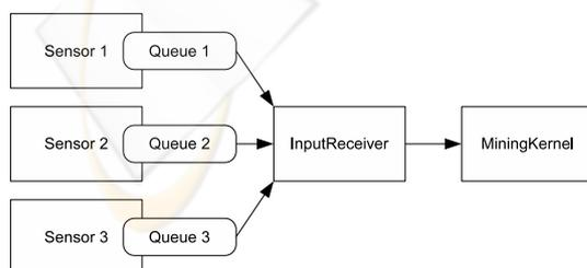
Figure 1: Threaded classes in the framework are illustrated as rectangular boxes. Arrows illustrate data flow within the framework. The boxes with rounded corners represent data buffers of the sensors.
