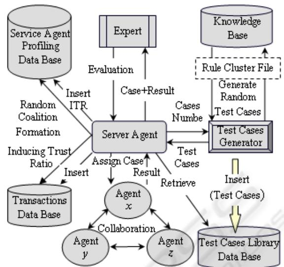
Figure 1: Overall structure of the TCGM.
