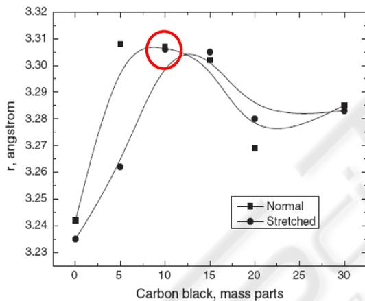
Figure 5: Mean radius of free volume cavities in PNCC as a function of carbon black content in normal and stretched ( $\Delta l = 15$  mm) states measured by PALS.
