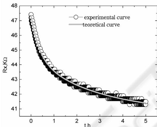
Figure 3: Electrical resistance relaxation of specimen in open air. The sample was exhibited to tetrahydrofuran for 30s.
