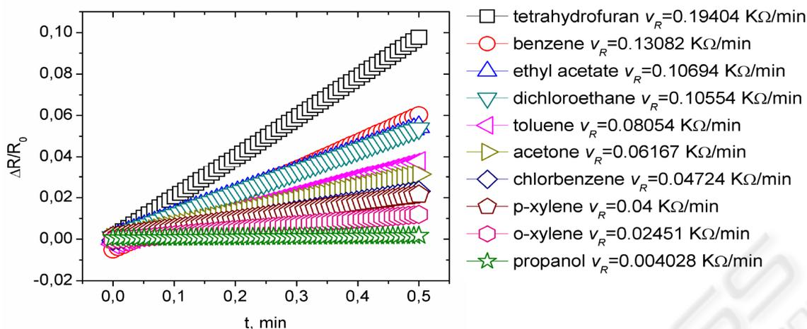
Figure 1: The change of relative resistance vs. time for the sample, held in saturated vapours of different solvents.
