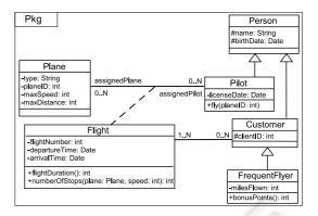
Figure 1: Example of a UML class diagram.
