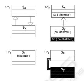
Figure 5: UML positive and negative constraints.
