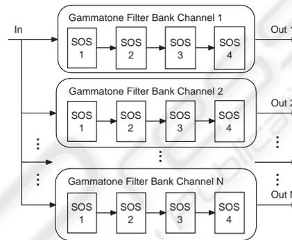
Figure 2: Slaney's digital Gammatone filter bank.
