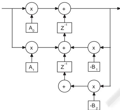
Figure 5: A second-order section of the Gammatone filter.
