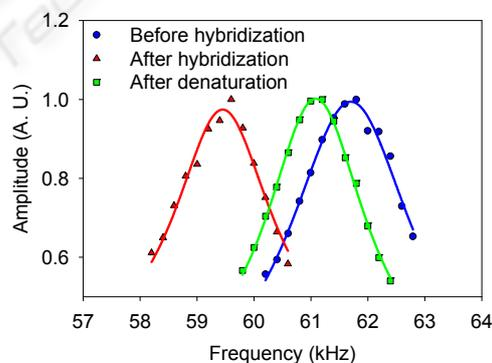
Figure 3: Dynamic response of cantilever to DNA hybridization and denaturation.
