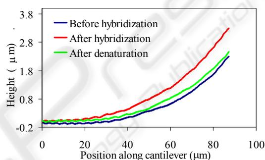
Figure 2: Static response of cantilever to complementary DNA hybridization and denaturation.
