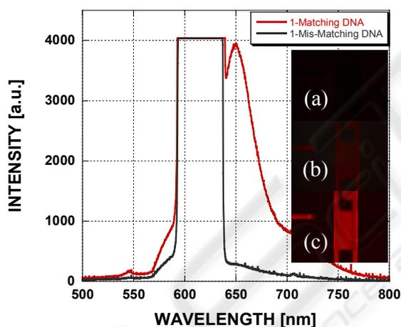
Figure 6: Collected output spectra demonstrating successful DNA hybridization. Inset: fluorescence microscope images of device: (a) after probe DNA attachment (b) after mismatching target DNA (c) after exposure to matching target DNA.
