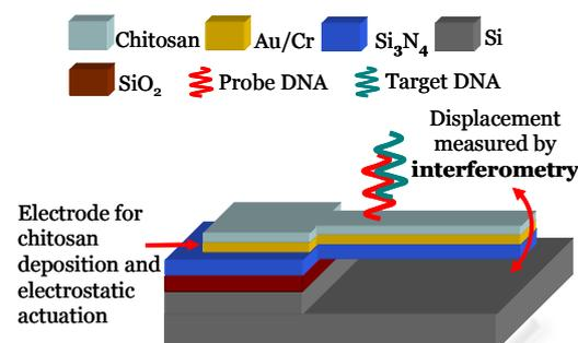
Figure 1: Cross sectional schematic of microcantilever sensor.
