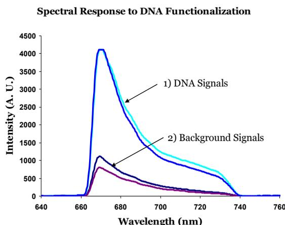
Figure 5: Spectra of optical emission signals received both 1) after introduction of fluorescent DNA and 2) when no fluorophores are present.
