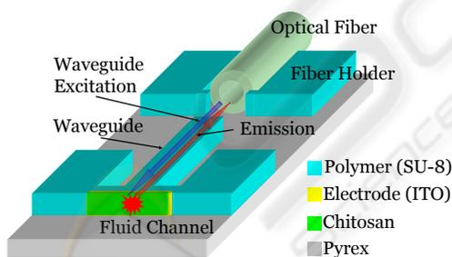
Figure 4: Schematic of the optical biosensor.
