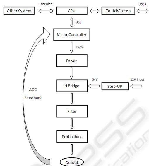
Figure 4: Block Diagram of the device internal structure and the links between the various sub-systems.
