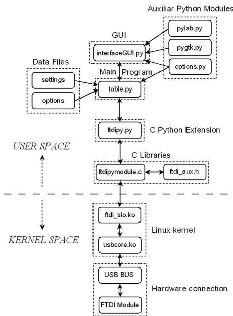
Figure 2: Software structure.
