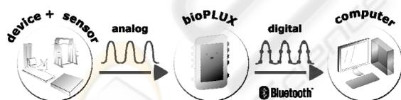
Figure 2: Schematic representation of powerPlux hardware.
