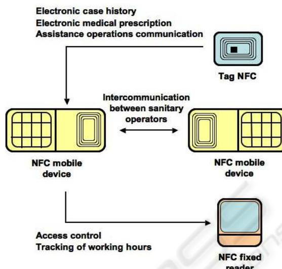
Figure 2: NFC applications in sanitary environment.
