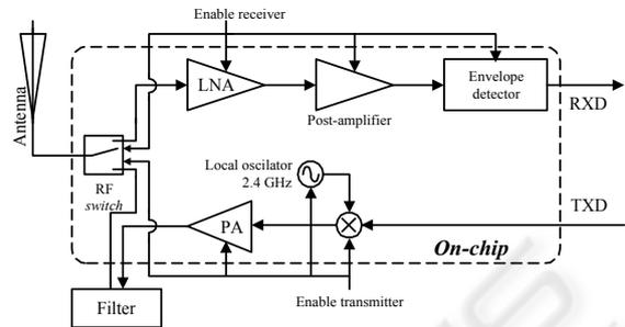
Figure 3: The block schematic of the transceiver.
