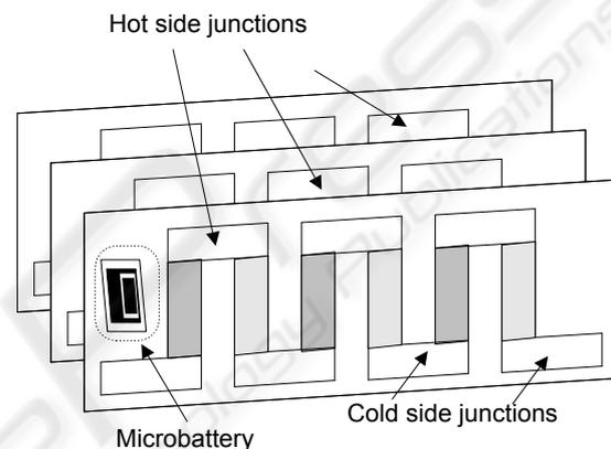
Figure 1: An artist impression of a thermoelectric microdevice.
