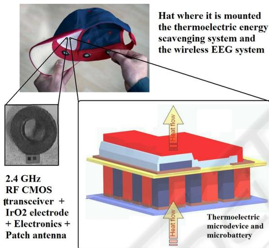
Figure 5: An artist impression of the thermoelectric scavenging system and an wireless EEG module.
