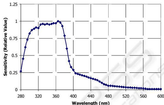
Figure 1: Spectral sensitivity characteristics of the ML8511.
