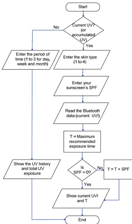
Figure 3: Software operation (it receives the new UV index each 15 seconds and stores to average for each hour).
