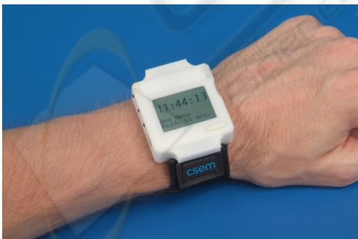
Figure 1: Wrist fall detection system.
