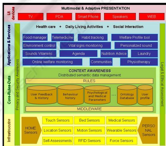
Figure 1: AmIE service system – building blocks.
