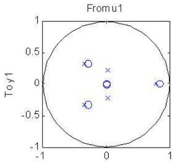
Figure 13: Poles and zeroes of the model for the channel between PC2 and PC5.
