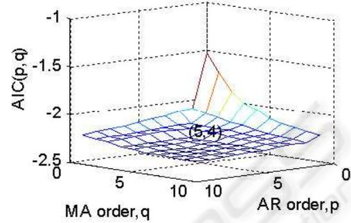
Figure 6: Order identification for acupoint signal using AIC.
