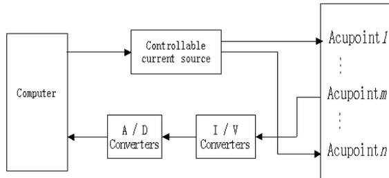
Figure 1: Acupoint signal measuring method using three-electrodes.
