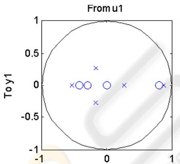
Figure 10: Poles and zeroes of the model for the channel between LU3 and non-acupoint 1.
