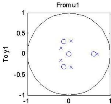
Figure 9: Poles and zeroes of the model for the channel between LU3 and LU5.
