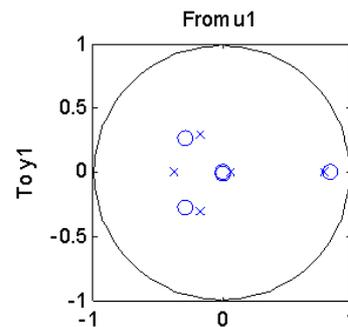
Figure 12: Poles and zeroes of the model for the channel between PC2 and PC4.
