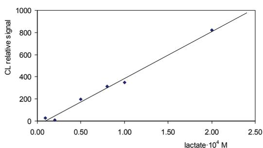
Figure 6: Linear calibration of lactate biosensor.
