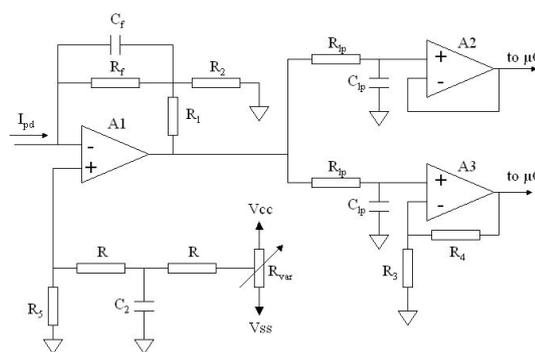
Figure 3: Measurement circuit.
