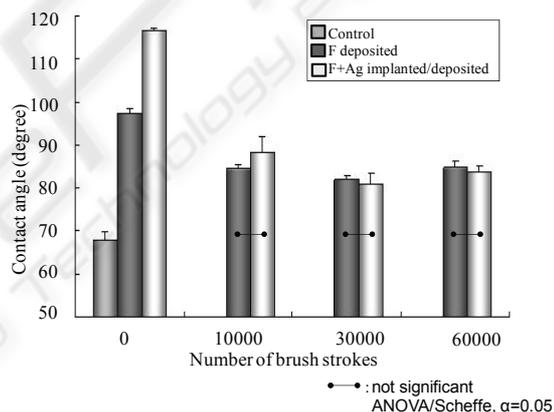
Figure 3: Contact angles of distilled water on the F deposited and F+Ag implanted-deposited PMMA before/after the brushing abrasion test. Horizontal lines indicate no significant differences (ANOVA/ Scheffe,  $\alpha = 0.05$ ).
