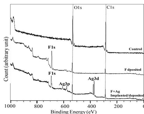
Figure 1: XPS wide-scan spectra of PMMA specimens.
