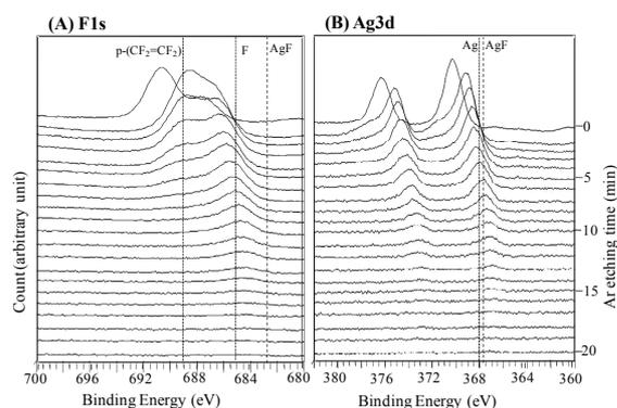
Figure 2: F1s (A) and Ag3d (B) XPS depth profiles of the F+Ag implanted-deposited PMMA. Dashed lines show the binding energy value of p-(CF<sub>2</sub>=CF<sub>2</sub>): 689.0 eV, F: 685 eV and AgF: 682.7 eV in the F1s depth profile (A), and Ag: 368.2 eV and AgF: 367.7 eV in the Ag3d depth profile (B). The values were based from Briggs and Seah, (1990).
