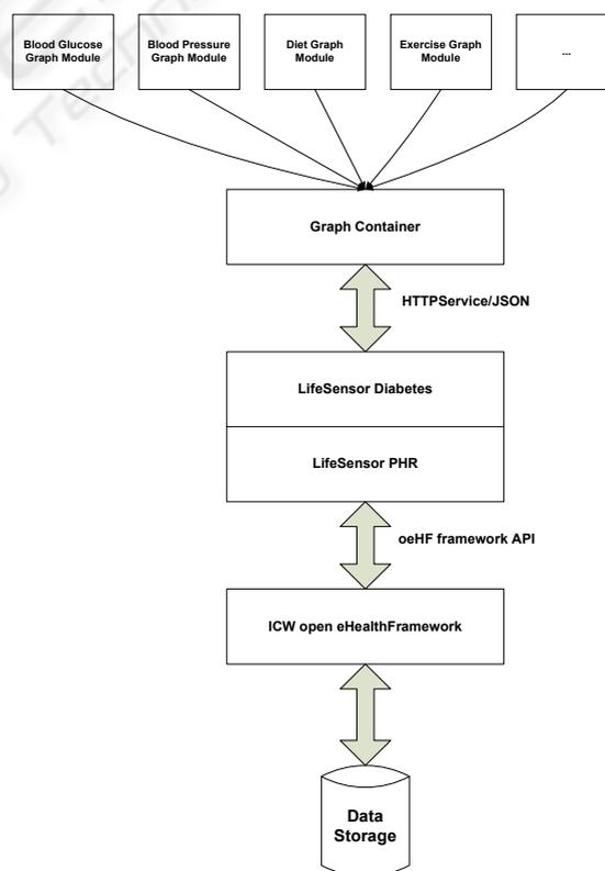
Figure 3: Module integration with LifeSensor.
