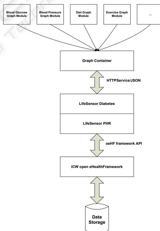
Figure 3: Module integration with LifeSensor.
